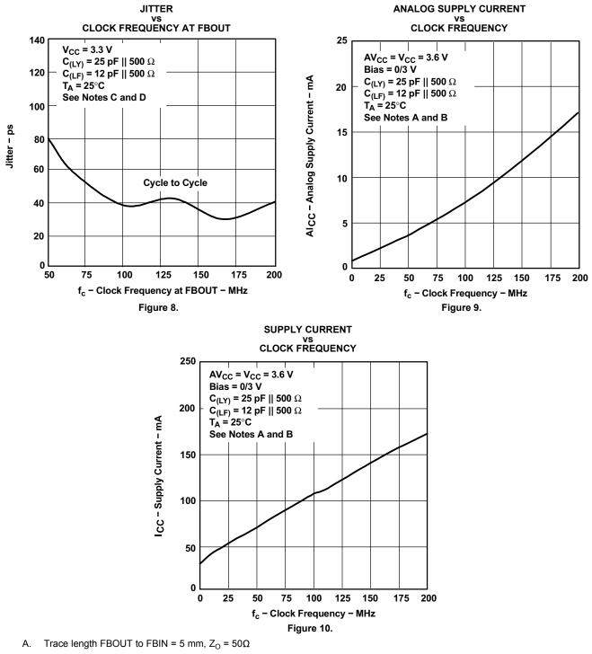
B.  $C_{(LY)}$  = Lumped capacitive load  $Y_{1-n}$
