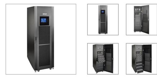
3-phase 20kVA UPS system offers network-grade power protection in a highly configurable, modular and scalable medium-chassis rack-width frame. Internal battery module can support a full load up to 3.9 minutes.
