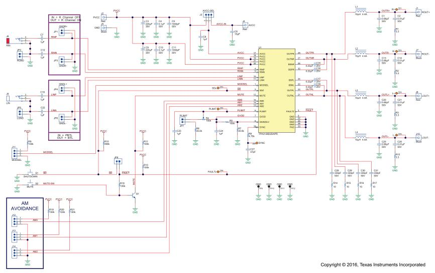
Figure 4. TPA3128D2EVM Schematic
