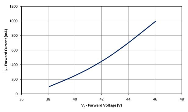
Figure 6: Typical forward current vs. forward voltage @  $T_c = 25^{\circ}C$ .
