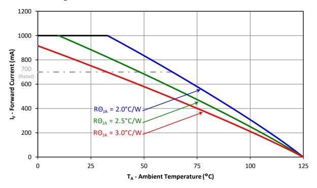
Figure 11: Maximum forward current vs. ambient temperature based on  $T_{J(MAX)}$  = 125°C.
