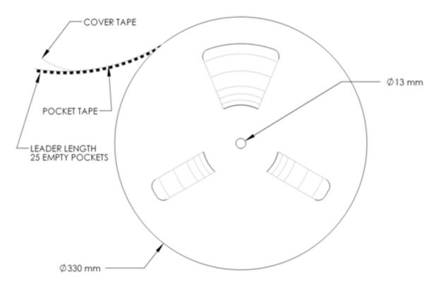
Figure 13: Emitter Reel specifications (mm).
