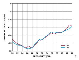
Figure 17. Output Return Loss vs. Frequency for Various  $V_{DD}$ ,  $I_{DQ}$  = 1200 mA
