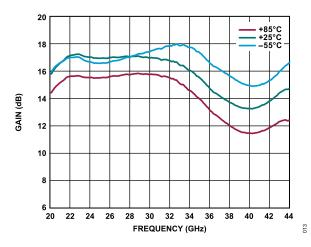
Figure 13. Gain vs. Frequency for Various Temperatures,  $V_{DD}$  = 5 V,  $I_{DQ}$  = 1200 mA
