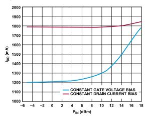
Figure 59.  $I_{DD}$  vs. RF Input Power ( $P_{IN}$ ),  $V_{DD}$  = 5 V, Frequency = 32 GHz for Constant Drain Current Bias and Constant Gate Voltage Bias
