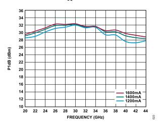
Figure 23. P1dB vs. Frequency for Various  $I_{DQ}$ ,  $V_{DD}$  = 5 V
