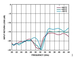
Figure 12. Input Return Loss vs. Frequency for Various Temperatures,  $V_{DD}$  = 5 V,  $I_{DQ}$  = 1200 mA
