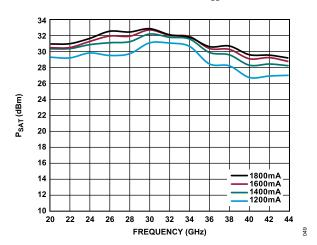
Figure 49.  $P_{SAT}$  vs. Frequency for Various Drain Currents,  $V_{DD}$  = 5 V, Data Measured with Constant  $I_{DD}$
