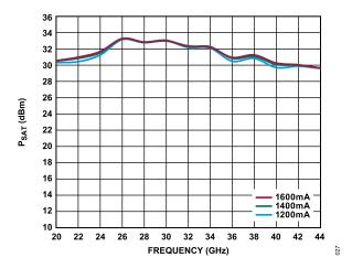
Figure 27.  $P_{SAT}$  vs. Frequency for Various  $I_{DQ}$ ,  $V_{DD}$  = 5 V
