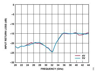
Figure 15. Input Return Loss vs. Frequency for Various  $V_{DD}$ ,  $I_{DQ}$  = 1200 mA
