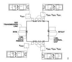
Figure 64. Assembly Diagram
