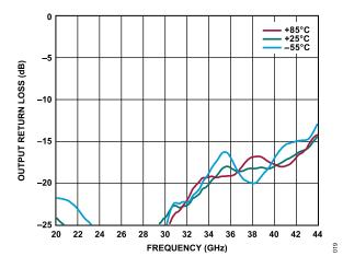
Figure 19. Output Return Loss vs. Frequency for Various Temperature,  $V_{DD}$  = 5 V,  $I_{DQ}$  = 1200 mA
