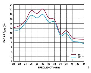
Figure 31. PAE at  $P_{SAT}$  vs. Frequency for Various  $V_{DD}$ ,  $I_{DQ}$  = 1200 mA, PAE Measured at  $P_{SAT}$
