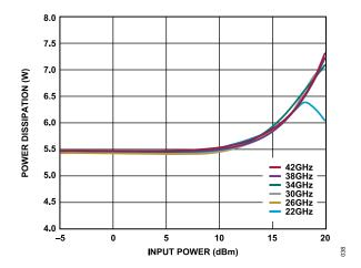
Figure 38. Power Dissipation vs. Input Power at T = 85°C,  $V_{DD}$  = 5 V,  $I_{DD}$  = 1200 mA
