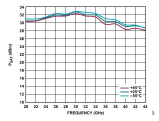
Figure 47.  $P_{SAT}$  vs. Frequency for Various Temperatures,  $V_{DD}$  = 5 V, Data Measured with Constant  $I_{DD}$
