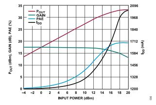
Figure 30. P<sub>OUT</sub>, Gain, PAE, and Power PAE, Drain Current with RF Applied (I<sub>DD</sub>) vs. Input Power, 26 GHz, V<sub>DD</sub> = 5 V, I<sub>DD</sub> = 1200 mA
