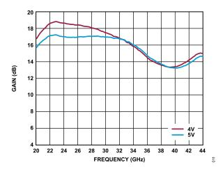
Figure 11. Gain vs. Frequency for Various  $V_{DD}$ ,  $I_{DQ}$  = 1200 mA
