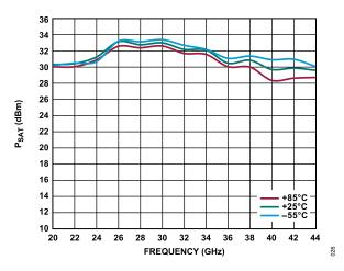
Figure 26.  $P_{SAT}$  vs. Frequency for Various Temperatures,  $V_{DD}$  = 5 V,  $I_{DQ}$  = 1200 mA
