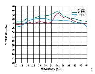
Figure 36. Output IP3 vs. Frequency for Various Temperatures,  $P_{OUT}$  per Tone = 14 dBm,  $V_{DD}$  = 5 V,  $I_{DQ}$  = 1200 mA
