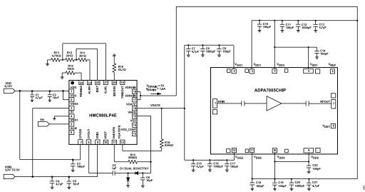
Figure 55. Application Circuit using HMC980LP4E with ADPA7005CHIP
