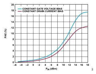
Figure 61. PAE vs.  $P_{IN}$ ,  $V_{DD}$  = 5 V, Frequency = 32 GHz, Constant Drain Current Bias and Constant Gate Voltage Bias
