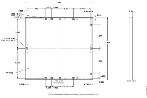
Figure 65. 12-Pad Bare Die [CHIP] (C-12-3) Dimensions shown in millimeters
