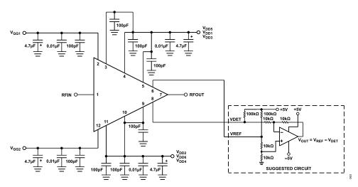
Figure 63. Typical Application Circuit Using the HMC980LP4E with the ADPA7005CHIP
