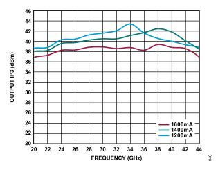
Figure 40. Output IP3 vs. Frequency for Various  $I_{DQ}$ ,  $P_{OUT}$  per Tone = 14 dBm,  $V_{DD}$  = 5 V
