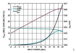
Figure 37.  $P_{OUT}$ , Gain, PAE, and  $I_{DD}$  vs. Input Power, 38 GHz,  $V_{DD}$  = 5 V,  $I_{DD}$  = 1200 mA
