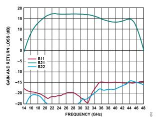
Figure 10. Gain and Return Loss vs. Frequency,  $V_{DD}$  = 5 V,  $I_{DQ}$  = 1200 mA
