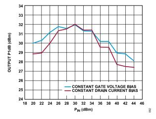
Figure 62. Output P1dB vs.  $P_{IN}$ ,  $V_{DD}$  = 5 V, Frequency = 32 GHz, Constant Drain Current Bias and Constant Gate Voltage Bias
