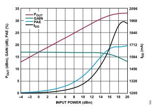
Figure 33.  $P_{OUT}$ , Gain, PAE, and  $I_{DD}$  vs. Input Power, 30 GHz,  $V_{DD}$  = 5 V,  $I_{DD}$  = 1200 mA
