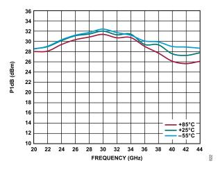
Figure 22. Output P1dB vs. Frequency for Various Temperatures,  $V_{DD}$  = 5 V,  $I_{DQ}$  = 1200 mA
