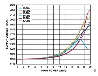
Figure 42. Supply Current  $I_{DD}$  vs. Input Power at Various Frequencies,  $V_{DD}$  = 5 V,  $I_{DD}$  = 1200 mA
