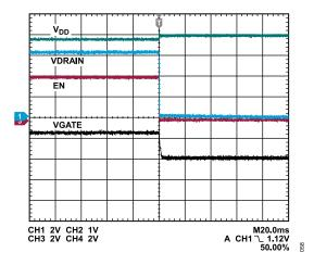
Figure 58. Turn Off HMC980LP4E Outputs to ADPA7005CHIP
