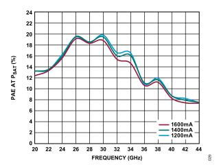
Figure 29. PAE at  $P_{SAT}$  vs. Frequency for Various  $I_{DQ}$ ,  $V_{DD}$  = 5 V,  $I_{DQ}$  = 1200 mA, PAE Measured at  $P_{SAT}$
