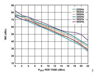
Figure 43. IM3 Distortion Relative to Carrier vs.  $P_{OUT}$  per Tone,  $V_{DD}$  = 5 V,  $I_{DQ}$  = 1200 mA
