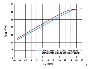
Figure 60. P<sub>OUT</sub> vs. P<sub>IN</sub>, V<sub>DD</sub> = 5 V, Frequency = 32 GHz, Constant Drain Current Bias and Constant Gate Voltage Bias
