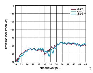
Figure 18. Reverse Isolation vs. Frequency for Various Temperatures,  $V_{DD}$  = 5 V,  $I_{DQ}$  = 1200 mA
