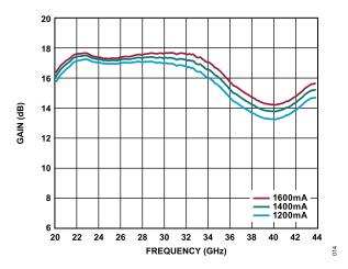
Figure 14. Gain vs. Frequency for Various  $I_{DQ}$ ,  $V_{DD}$  = 5 V
