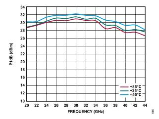
Figure 46. P1dB vs. Frequency for Various Temperatures,  $V_{DD}$  = 5 V, Data Measured with Constant  $I_{DD}$
