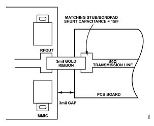
Figure 53. High Frequency Output Wideband Matching
