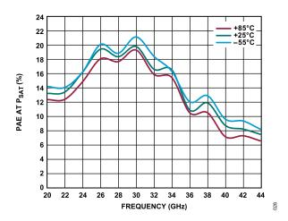
Figure 28. Power Added Efficiency (PAE) at  $P_{\rm SAT}$  vs. Frequency for Various Temperatures,  $V_{DD}$  = 5 V,  $I_{DQ}$  = 1200 mA, PAE Measured at  $P_{\rm SAT}$
