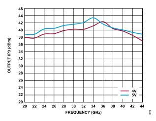
Figure 39. Output IP3 vs. Frequency for Various  $V_{DD}$ ,  $P_{OUT}$  per Tone = 14 dBm,  $V_{DD}$  = 5 V,  $I_{DQ}$  = 1200 mA
