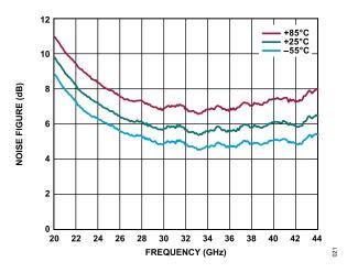
Figure 21. Noise Figure vs. Frequency for Various Temperatures,  $V_{DD}$  = 5 V,  $I_{DQ}$  = 1200 mA
