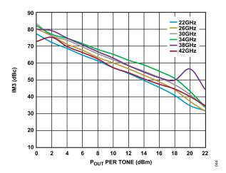
Figure 44. Third-Order Intermodulation (IM3) Distortion Relative to Carrier vs.  $P_{OUT}$  per Tone,  $V_{DD} = 4 \text{ V, } I_{DQ} = 1200 \text{ mA}$
