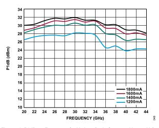
Figure 48. P1dB vs. Frequency for Various Drain Currents,  $V_{DD}$  = 5 V, Data Measured with Constant  $I_{DD}$
