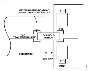
Figure 52. High Frequency Input Wideband Matching
