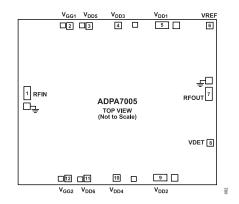
Figure 2. Pin Configuration
